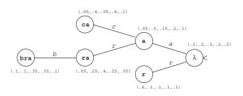
**Fig. 1.** An example of a PST over the alphabet  $\Sigma = \{a, b, c, d, r\}$ . The string inside each node is a memorized suffix and the adjacent vector is its probability distribution over the next symbol. (e.g. since suf<sub>T</sub>(bacara) = ra, the probabilities  $P_T(?|bacara) = \{0.05, 0.25, 0.4, 0.25, 0.05\}$  for  $\{a, b, c, d, r\}$  respectively).
